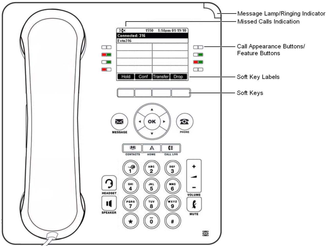
The phone supports 24 programmable call appearance/feature buttons. The labels for these are displayed in the main display and can be controlled by the adjacent buttons.
