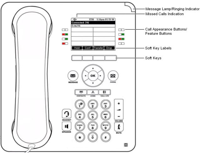
The phone supports 24 programmable call appearance/feature buttons. The labels for these are displayed in the main display and can be controlled by the adjacent buttons.
