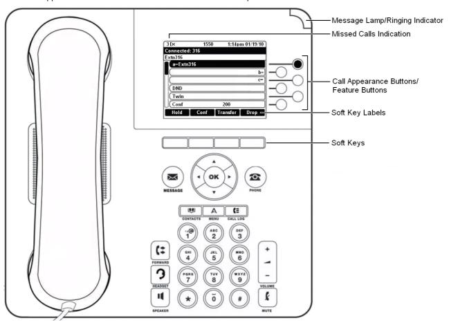
This phone supports 24 programmable call appearance/feature buttons. The labels for 6 of these buttons are visible on the main display and can be controlled by the adjacent buttons to the right. You can use the ▲ up and down ▼ arrow keys to scroll the display. You can also use the ◀ left and right ▶ arrow keys to move through the button features in pages of 6.
